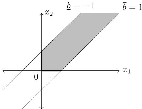
**Figure 6.2:** The feasible set (gray) and the set of optimal solutions (thick black) of ILP (38).
