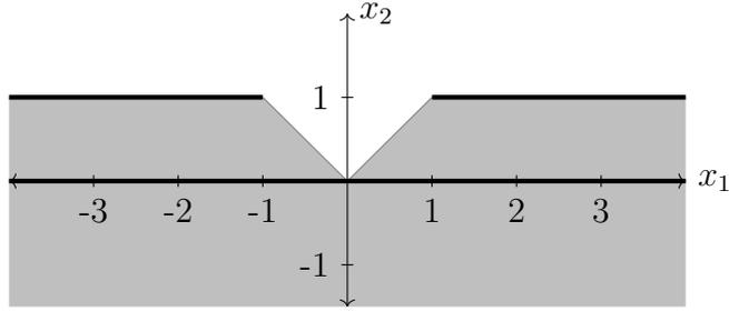
**Figure 5.1:** The union of all feasible sets (gray) and the set of all optimal solutions (thick black) of ILP (26).
