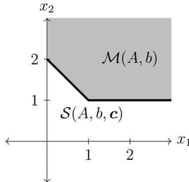
**Figure 2.2:** The feasible set (gray) and the set of optimal solutions (thick black) of ILP (1).
