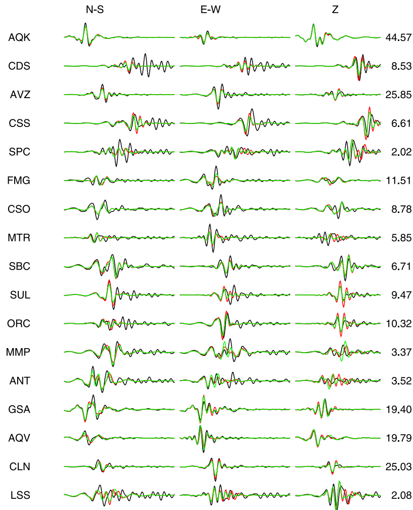
Figure 4. Comparison between observed (black) and synthetic displacements for the L'Aquila event (green for the TSVD approach, red for the best fitting MuFEx model shown in Figure 5a). The records are band-pass filtered in the range of 0.06–0.30 Hz and have a duration of 100 s. The maximum amplitudes of the observed records in mm are shown as numbers.
