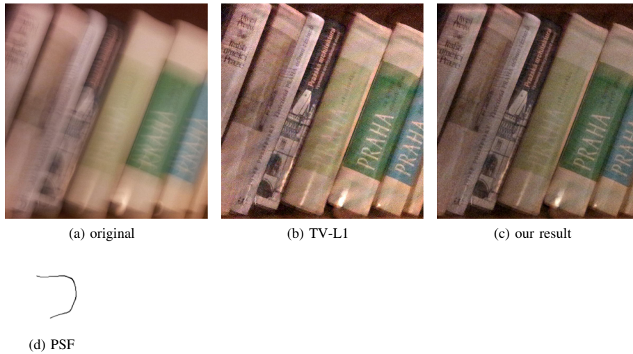
Fig. 5 Test 3: 1/2 s exposure, 72 × 76 estimated PSF.
