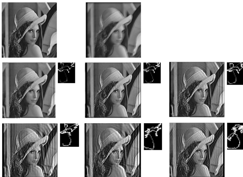
Fig. 8 Noise in gyroscope data. Synthetically blurred Lena image using PSF from recorded gyroscope samples and afterward deblurred using PSF from measurements with variable amount of noise. Images are from left to right, top to bottom: original, blurred, and six deblurred images using original gyroscope data altered by random Gaussian noise with variance from 0 to 0.05 (gyroscope measurements are in rad/s).
