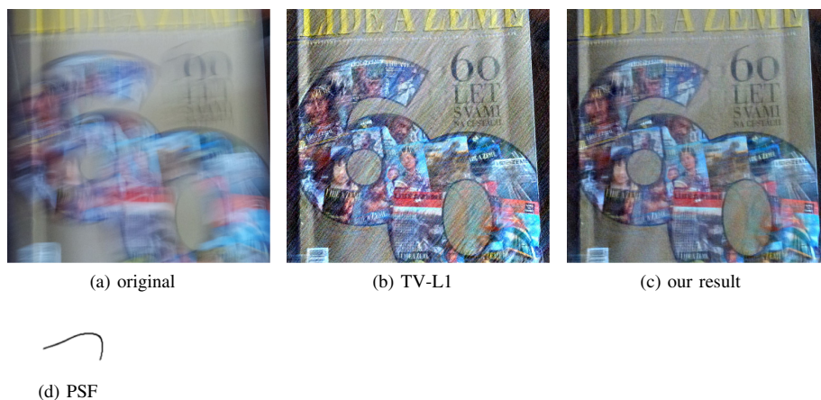
Fig. 4 Test 2: 1/9 s exposure, 21 \times 28 estimated PSF.
