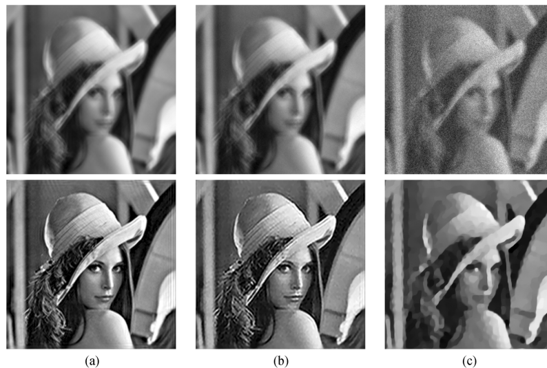
Fig. 11. Estimated sharp images for the PSF size set to 21 \times 21 and three different noise levels: (a) 50, (b) 30, and (c) 10 dB. Results are arranged as in Fig. 10. The first row shows one of the input images and the second row shows the estimated image. (a) 50 dB. (b) 30 dB. (c) 10 dB.
